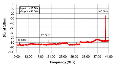
The Equalizer micrometer adjusts the amplitude of one pulse leg so that the two recombined pulses have equal amplitude. The suppression of the input frequency is at least 35 dB.
