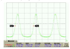
The Sync micrometer precisely adjusts the pulse time delay in one leg to the desired value. The maximum tunable pulse delay is 70 ps.
